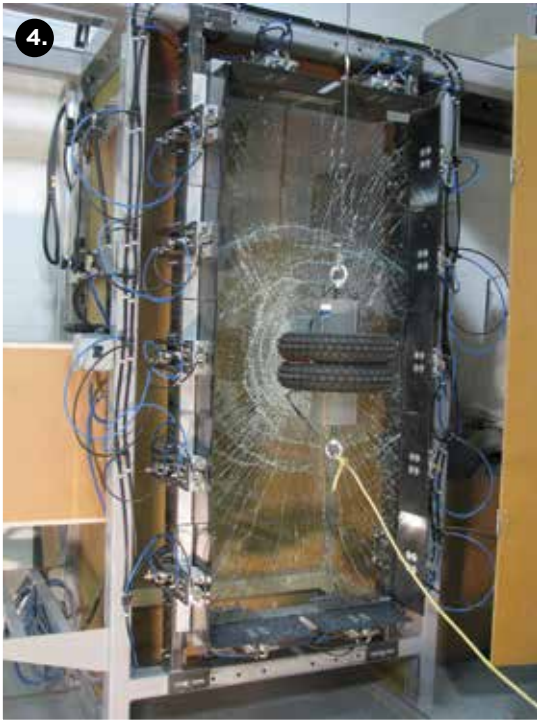
1. Blast resistance testing is shown here using a shock tube per ASTM F1642, F2927, and GSA-TS01. 2. Windborne debris testing for hurricane prone areas per TAS 201 and ASTM E1886/E1996–Large Missile Impact Test. 3. Lab staff demonstrate ASTM F3038 time evaluation of forced entry resistant systems. 4. Safety glazing testing per North American and European standards (picture is European standard). 5. Ballistics resistant testing per UL 752, NIJ0108.01, EN 1063, and DOS SD-STD-01.01.
